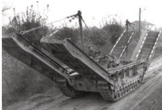
Churchill AVRE Mk III Armoured Ramp Carrier ('ARK'). It could bridge a 15 m gap, cope with 1.5 m of water, and be used in tandem.
