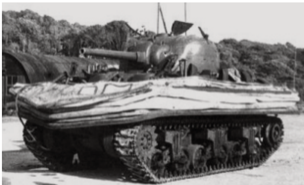
Sherman DD tank (skirt in stowed position).
