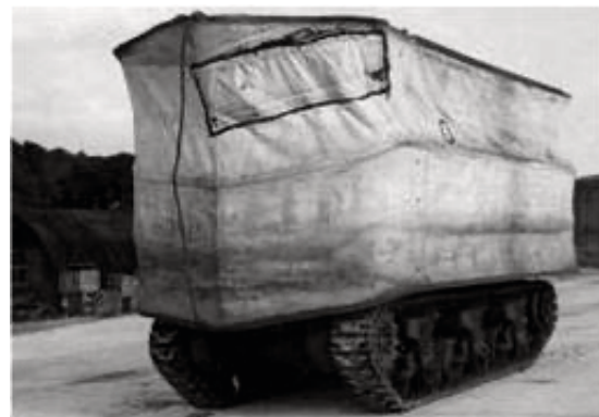
Sherman DD tank (skirt erected).
