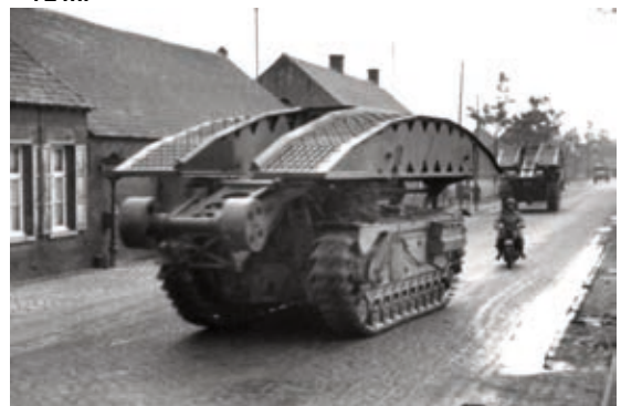
Churchill AVRE Mk III with No 2 Tank Bridge. It provided MLC 60(T) or MLC 40(W) crossing over a 9 m gap. Launch time was 90 seconds.
