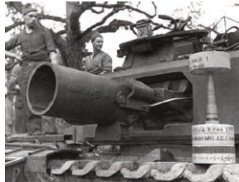
The 290 mm Petard spigot mortar. It could fire a 40 lb charge (called a 'Dustbin') up to 72 m.
